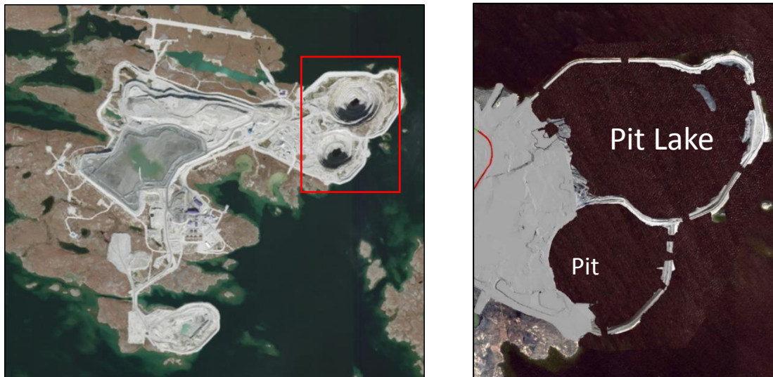
Figure 6: Diavik’s closure plan is to fill the pits with water to create pit lakes Photo courtesy of Diavik
